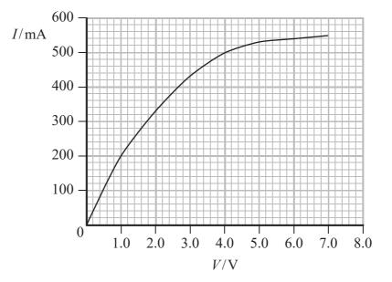
This filament lamp is connected across a battery of e.m.f. 6.0 V as shown below.
